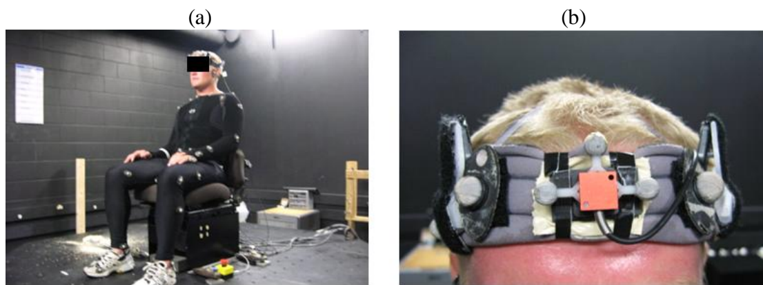
Figure 1.6 One participant seated on agriculture seat (a) where a head-mounted halo (b) was worn with an accelerometer and three markers attached.
